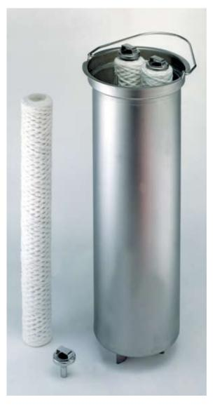
Flow is introduced from above and circulates around cartridges. Fluid flows through cartridge walls, leaving contaminant on media, and "clean" fluid exits through bottom outlet. B A G F I L T E R C O N V E R T E R
