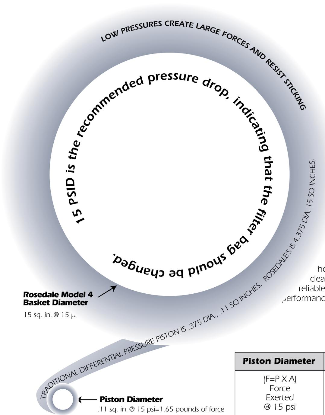
Most differential pressure indicators use a piston connected through a small hole in the side of the filter. This hole could clog, or the piston could easily be blocked or restricted. Rosedale's piston is much larger in diameter and surface area, requiring a greater blockage to restrict it, and since it is inside the housing, there is no outside hole to clog. It produces a cleaner, more accurate and reliable unit, providing excellent performance and value.
