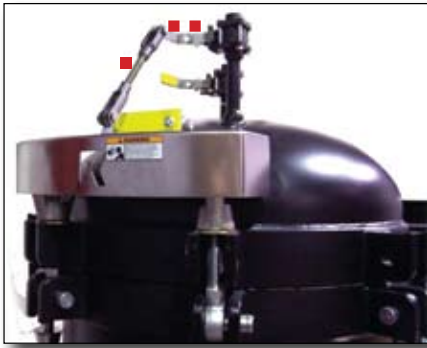
■ OPTIONAL PRESSURE RELEASE SAFETY ASSEMBLY - Must be opened prior to swing bolts. ■ ■ ■ PAD-LOCK VALVE - Prevents accidental release of pressure.
