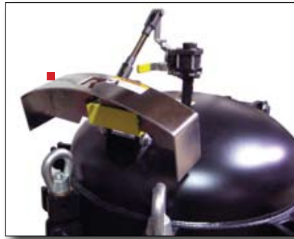
■ PRESSURE RELEASE SAFETY ASSEMBLY SHOWN IN OPEN POSITION - Opens vent valve and allows access to swing bolts.
