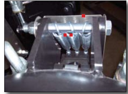
■ SPRING COVER ASSEMBLY - ■ ■ ■ COVER OPENING ASSIST SPRINGS -
