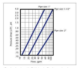
\*Based on housing only. Fluid viscosity, filter bag used, and expected dirt loading should be considered when sizing a filter.
