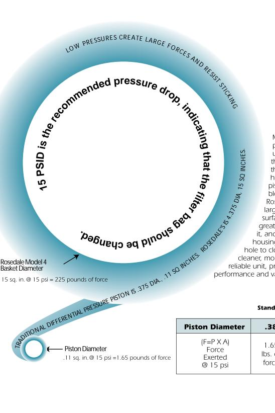
Most differential pressure indicators use a piston connected through a small hole in the side of the filter. This hole could clog, or the piston could easily be blocked or restricted. Rosedale's piston is much larger in diameter and surface area, requiring a greater blockage to restrict it, and since it is inside the housing, there is no outside hole to clog. It produces a cleaner, more accurate and reliable unit, providing excellent performance and value.
