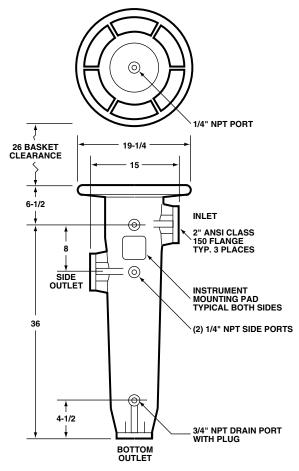
Dimensions are reference only and should not be used for hard plumbing. Consult factory for certified drawings.
