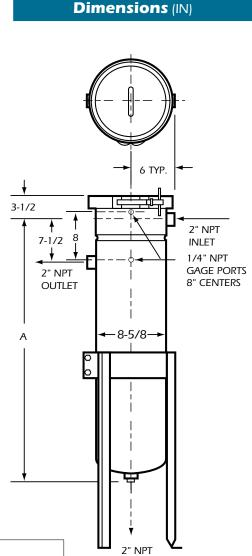
DRAIN OR OPTIONAL OUTLET 9/16 DIA. HOLES ON 12.0 DIA. BOLT CIRCLE
