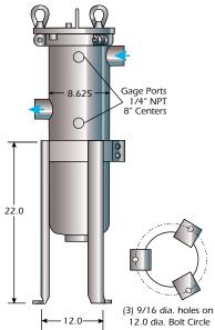
A clearance distance equal to basket depth must be available above housing for basket removal.
