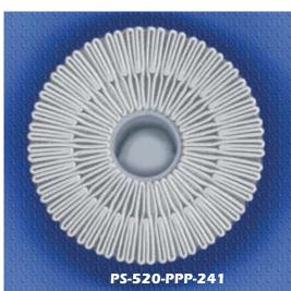
**2–**The PS-520-PPP-241 filters are manufactured in a "Y" pleat arrangement that optimizes physical size and maximizes effective surface area. The large surface area provides a low fluid flux rate maximizing dirt containment. This means element life is extended. NSF 61 listed.
