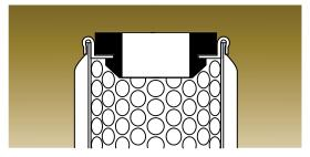
Rosedale seals are specially shaped to hold in place mechanically, like a grommet. There's little chance they will be dislodged and lost in handling. They are made in different thicknesses to provide seven different standard overall element lengths.
