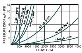
Recommended flow rates are based on housing only. Fluid viscosity, filter bag used, and expected dirt load should be considered when sizing a filter.
