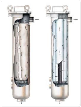
Pictured is a Model 6330. It can hold three 30-in. long cartridges (shown inserted) or a filter bag and support basket (at left). The two 3/4-in. ports at the bottom of the housing are 1) a dirty liquid drain (upper port), and 2) a clean liquid drain (lower port). The dirty liquid drain need not be used when filter bags are employed; if bags are properly removed, no dirt washes off downstream. (The use of a liquid displacer makes this easier to do.)
