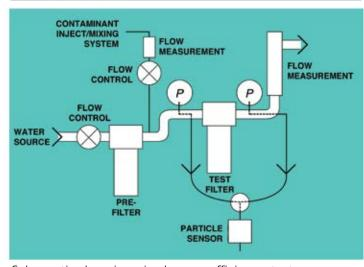
Schematic showing single-pass efficiency test
