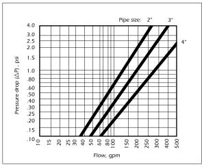
\*Based on housing only. Fluid viscosity, filter bag used, and expected dirt loading should be considered when sizing a filter.
