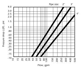
\*Based on housing only. Fluid viscosity, filter cartridge used, and expected dirt loading should be considered when sizing a filter.
