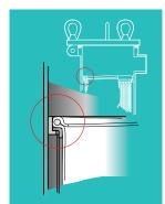
A single cover gasket is used to seal the opening, and covers can be installed and removed without tools.
