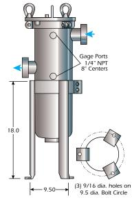
A clearance distance equal to basket depth must be available above housing for basket removal.
