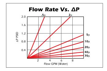
Flow rate is per single 10-inch element. For other liquid's, multiply the  $\Delta P$  by the fluid's viscosity in centipoise. For longer cartridges, divide the  $\Delta P$  by the number of 10-inch equivalents.
