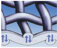
These elements are sintered at over 1100°C in a controlled atmosphere furnace. This process fuses metal molecules of the different layers at contact points into a new, completely integrated structure.
