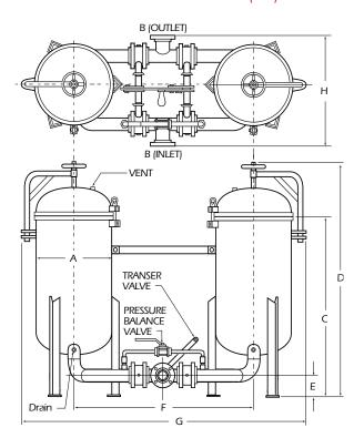
The inlets and outlets on all duplex systems come standard in a horizontal configuration (facing opposite directions). The option of arranging the inlet and outlet is available in three positions, 90° apart. The system is designed with flanged tees, allowing the orientation to be changed in the field.
