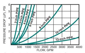
Based on housing only. Fluid viscosity, filter cartridge used, and expected dirt loading should be considered when sizing a filter.
