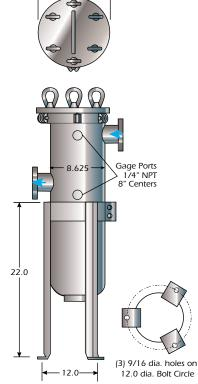
A clearance distance equal to basket depth must be available above housing for basket removal.
