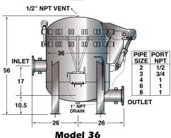
Dimensions are reference only and should not be used for hard plumbing. Consult factory for certified drawings.
