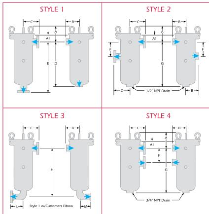
A clearance distance equal to basket depth must be available above housing for basket removal.
