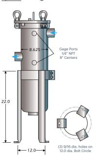
A clearance distance equal to the basket depth must be available above the housing for basket removal.
