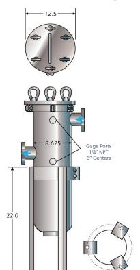
A clearance distance equal to the basket depth must be available above the housing for basket removal.
