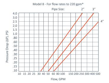
\*Based on housing only. Fluid viscosity, bag filter used, and expected dirt loading should be considered when sizing a filter.
