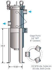
A clearance distance equal to the basket depth must be available above the housing for basket removal.
