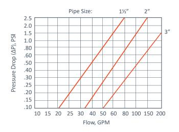
\*Based on housing only. Fluid viscosity, bag filter used, and expected dirt loading should be considered when sizing a filter.
