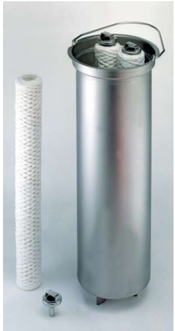
◀ Flow is introduced from above and circulates around cartridges. Fluid flows through cartridge walls, leaving contaminant on media, and "clean" fluid exits through bottom outlet.
